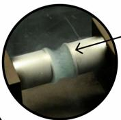
Oxygen trapped between magnets<sup>4</sup>
